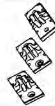
Style 1111F 1. Spot Face Drilling 2. Counter Bore Drilling 3. Counter Sink Drilling Nos. 1, 2, & 3 with or without rib bottom
