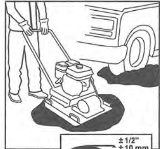
COMPACT. Use tamper, shovel, vibrating plate or wheel of a truck. Repair area should rise +/- 1/2" (13 mm) above road bed.
